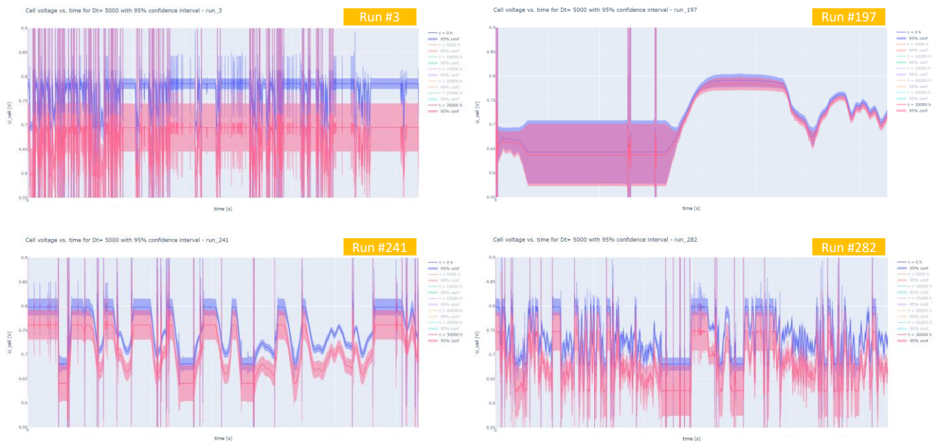
Figure 16. Voltage forecasting at t=0 and t=30000 h of the selected final model for simulation runs #3, #197, #241 and #252.
