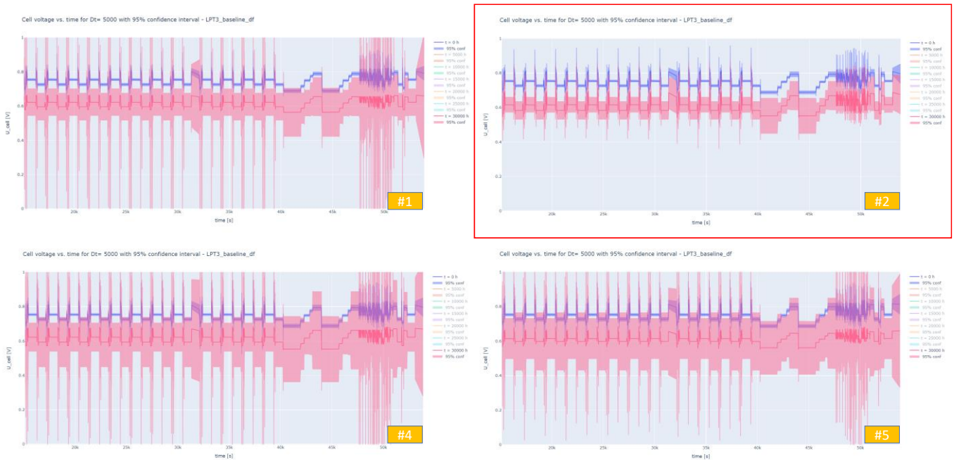
Figure 14. Confidence intervals of voltage forecasting in LPT1 at t=0 and t=30000 h, for four models of the table in Figure 11.
