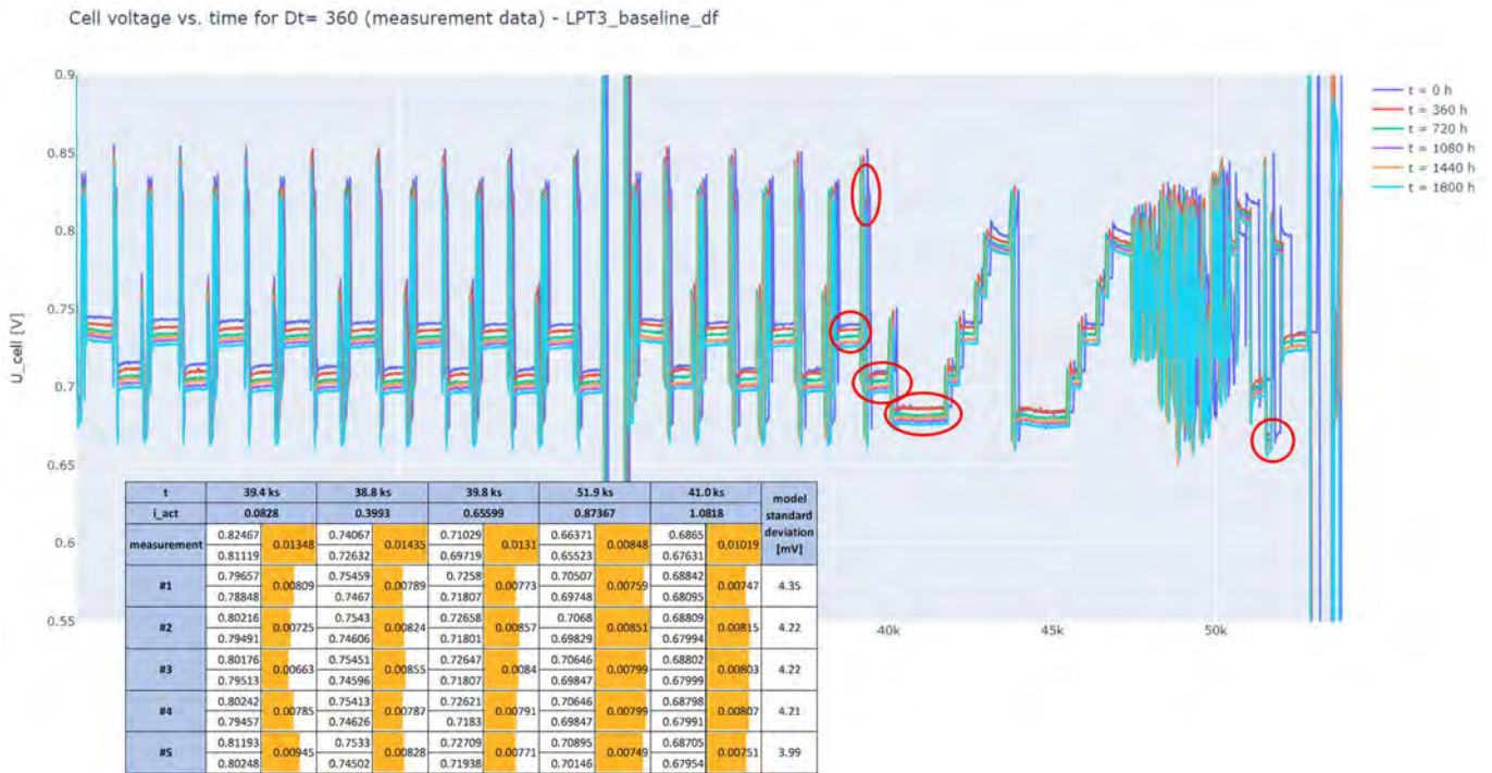
Figure 11. Fitting of various models on degradation trends. The table is showing the voltage drop in Volts at various current density levels (see also Figure 2) from t=0 to t=1800 h. The selected model is #2.
